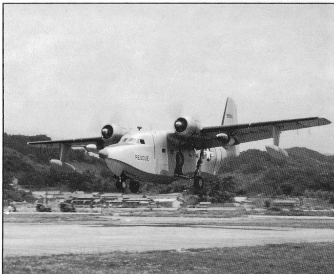
A 3rd ARS SA-16 takes off for another mission up the west coast of Korea in 1952. The SA-16 had a range of over 3000 miles, which meant it could fly to the mouth of the Yalu River, loiter for over an hour locating the downed pilot, then retrieve the pilot and bring him home. (credit-Budd Butcher)
